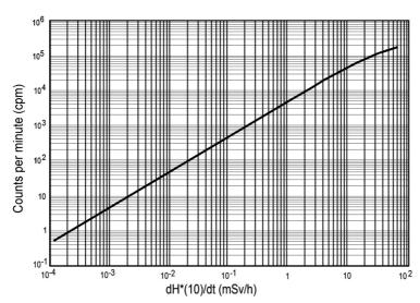
dH\*(10) / dt = Radiation dose equivalent rate for Cs-137 and Co-60 (mSv/h)
