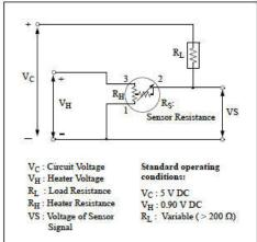
Fig 2. Standard circuit
