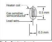
Fig 1a. Sensing element
