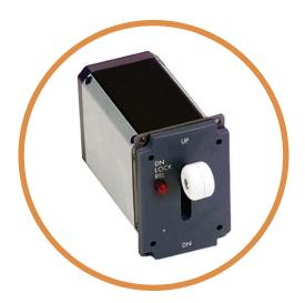
Operation of the control handle actuates six independently triggered SPDT (single pole, double throw) switches for signaling position status. A bank of 4-6 switches are triggered when the handle is moved from stowed position to down position or vice versa. The electrical signal initiate the deployment or retraction of the landing gear system.
