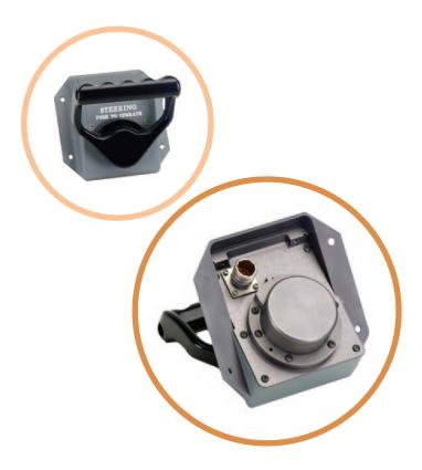
Operation of the steering handwheel downwardly actuates a single pole, double throw switch signaling that the handwheel is activated. A combination of this signal & the RVDT output is used to steer the nose landing gear left or right, during take off, landing and taxi.
