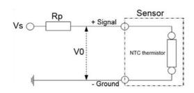
$Vs = 5V \pm 0.25V \\ Rp = 2.21k\Omega \pm 1\% \\ V0 = Measurement results based on RT curve$
