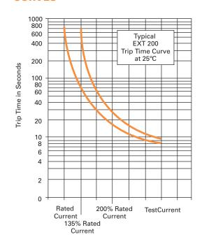
These curves are to be used only as a guide in selecting a protector for a particular application. Factors such as distance from the heat source and the method of mounting should be considered in selecting a protector. Final trip times are dependent upon terminal configuration and mounting in the application.
