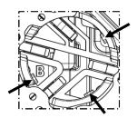
Locations to match when fitting the sensor (OX-04, CX-04)
