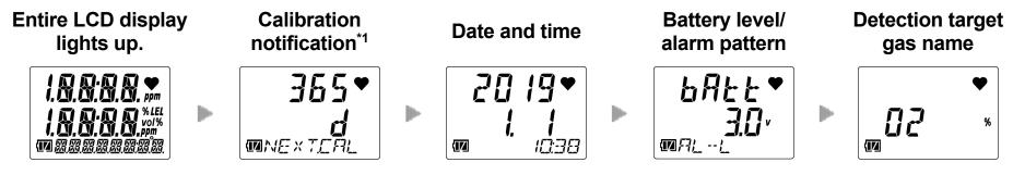
The buzzer blips once, and the power turns on.
