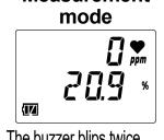
The buzzer blips twice, and the product switches to measurement mode \*3
