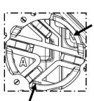
Locations to match when fitting the sensor (CO-04/HS-04/ SC-04 (SO2, NO2, HCN))
