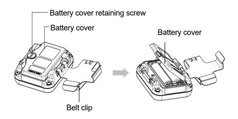
3 Remove the old batteries, then insert new batteries. Note the polarity.
