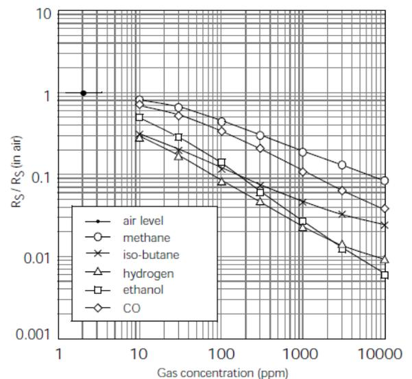
Fig3. Sensitivity characteristics
