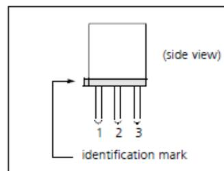
Fig 1c. Pin Layout
