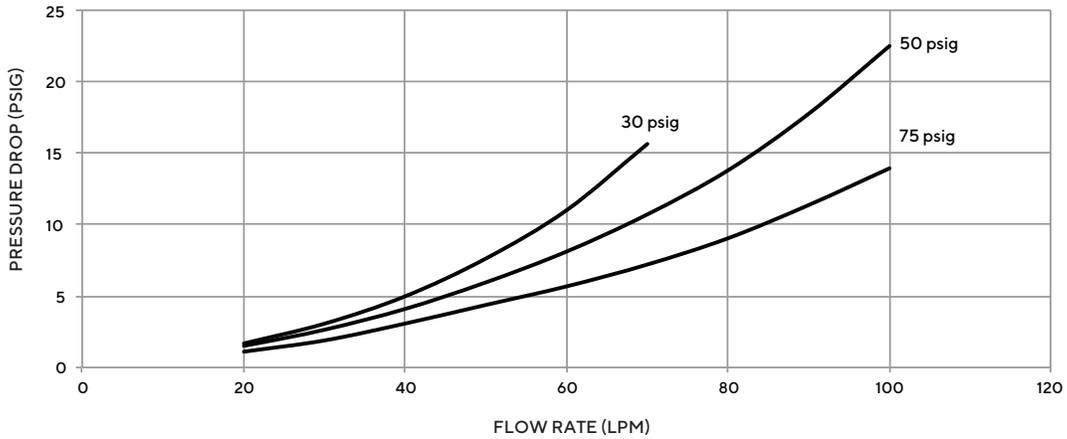
**Flow Rate -vs- Pressure Drop**
