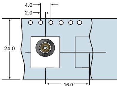
**DIMENSIONS FOR STANDARD PACKAGING OPTIONS (in millimeters)**
