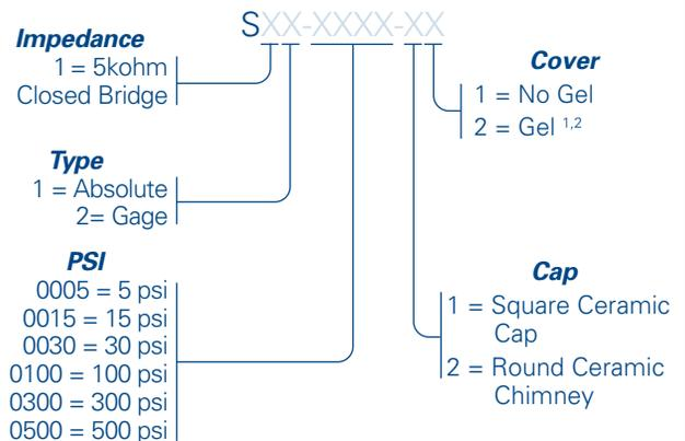
**Example:** S11-0015-11 offers 5kohm Impedance, Closed Bridge, Absolute Constraint, 15 psi, Square Ceramic Cap, No Gel
