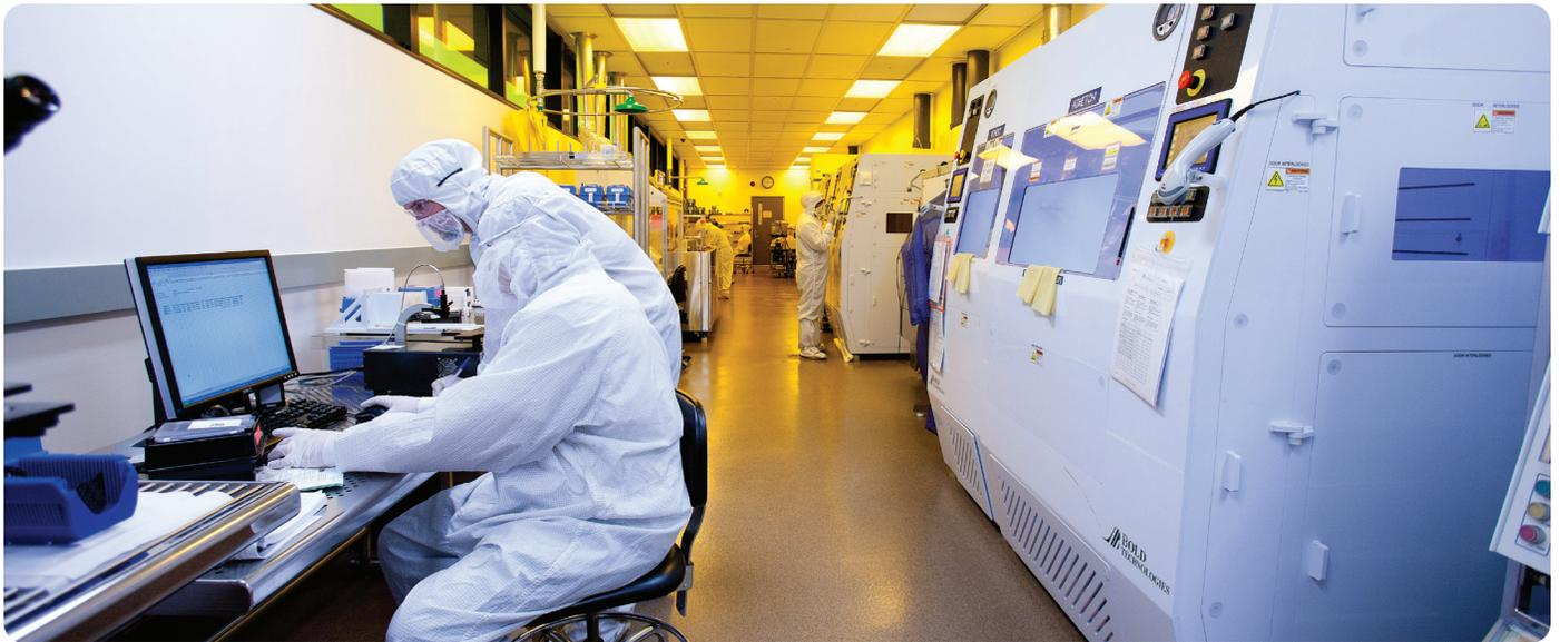
Merit Sensor owns and operates a MEMS wafer fab, which enables the production of customized piezoresistive pressure sensors.
