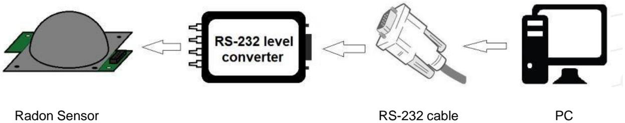
In order to connect the sensor to a micro controller or CPU that implements UART, the following scheme is recommended:
