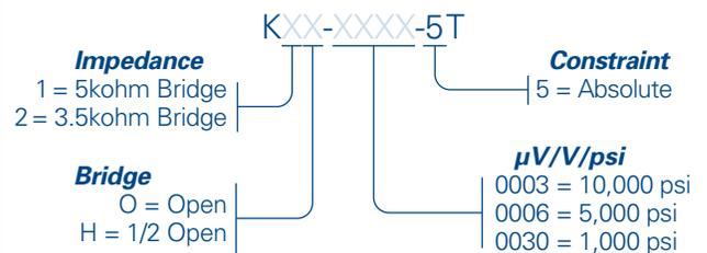
**Example:** K10-0003-5T offers 5kohm Impedance, Open Bridge, 10,000 psi and Absolute Constraint
